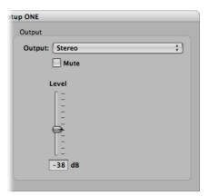
• Output pop-up menu: Determines the output gain. You can choose between Speaker/Headphone Out (Stereo) and Instrument Amp (Amp).
